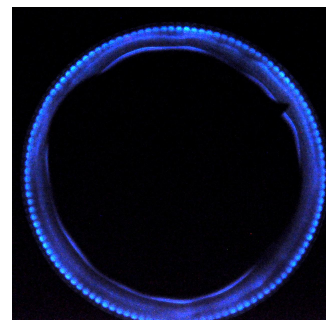
Figure 5: Pre-mixed flame of a T-140 anode and the respective Matlab representation. It is important to look at the exit plane flow to check for uniformity; in this case it is the flamelets around the edge.
