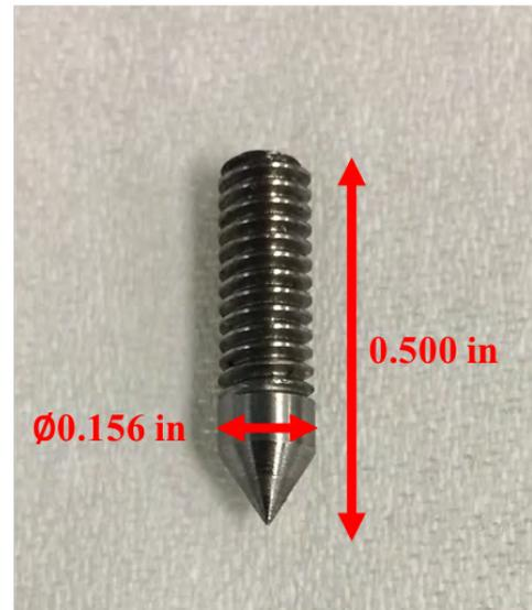
Figure 2.5: Needle electrode & supporting threaded rod.
