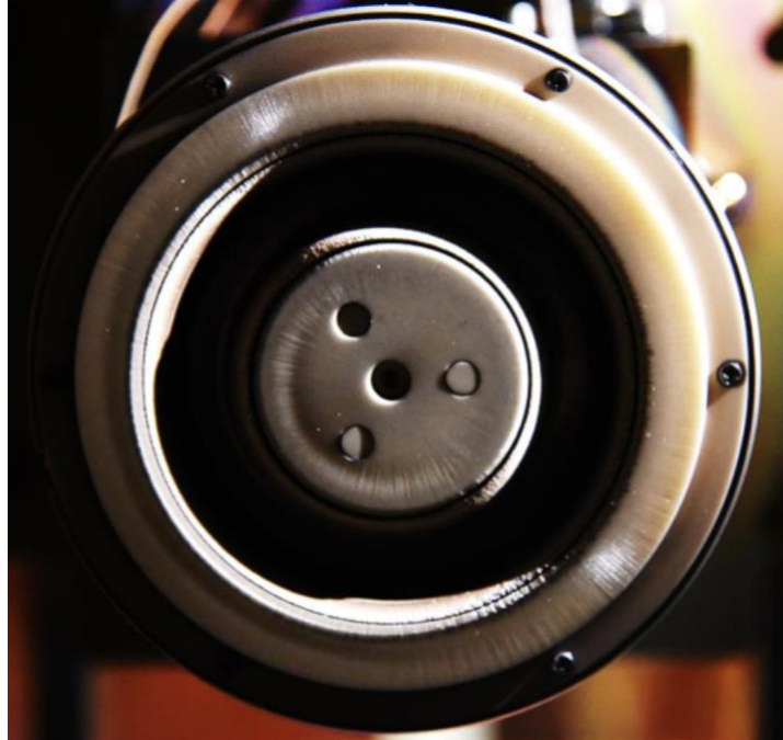
Figure 1: Photo of the NGHT-1X, a magnetically-shielded Hall-effect thruster, after 873 hours of operation during long-duration wear testing. Adapted from reference [8]
