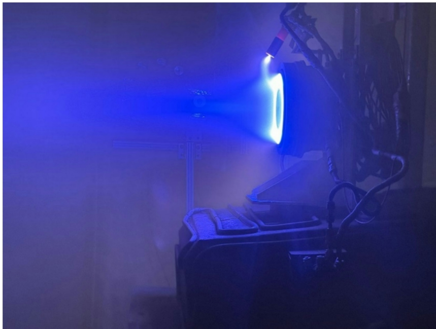
Fig. 1 T-140 operating on krypton at 300 V and 16 A
