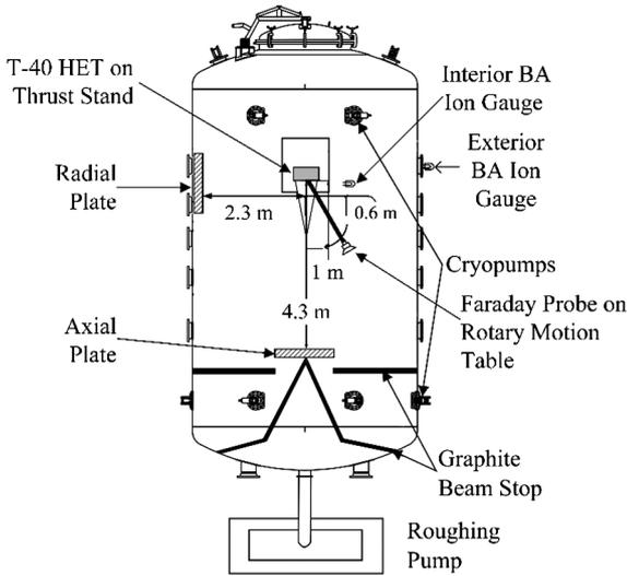
Fig. 1 Schematic of VTF-2 (not to scale).
