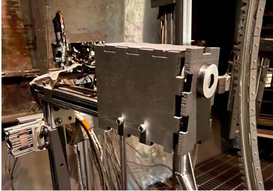
Figure 27 – RPA installed on VTF-2 radial arm for plume measurements
