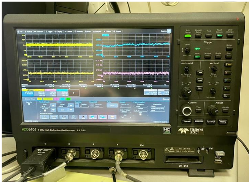
Figure 29 – Teledyne LeCroy HDO6104A oscilloscope used for the study.
