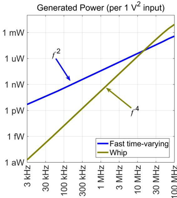
We have simulated our technique using an FDTD model of an antenna, and evaluated the current moment to determine the radiated power as a function of frequency.
