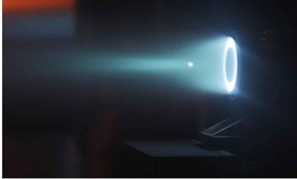
Figure 1: T-140 HET Operating in Vacuum Chamber. HET is operating with xenon propellant at a discharge voltage of 300 V and a discharge power of 3.1 kW. Ambient chamber pressure is 7.3 \times 10^{-6} Torr corrected for xenon.
