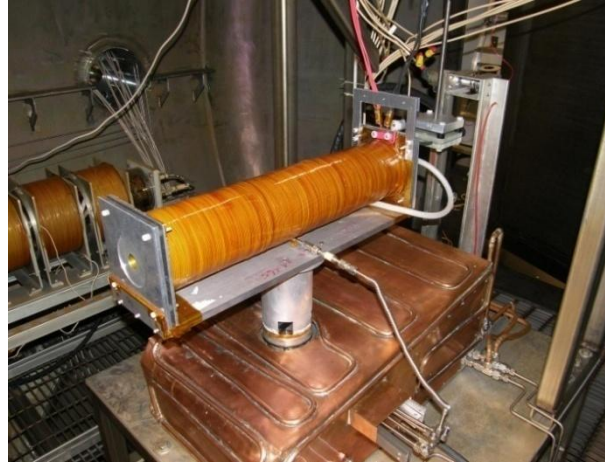
Figure 2. Medium-power helicon thruster mounted on thrust stand.
