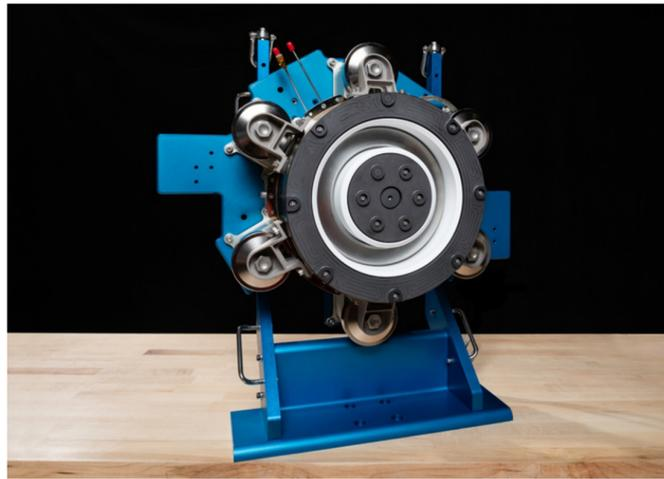
**Figure 8.** Magnetically-shielded Advanced Electric Propulsion System (AEPS) Engineering Test Unit 1. Image reprinted with permission from [11], NASA, 2019.
