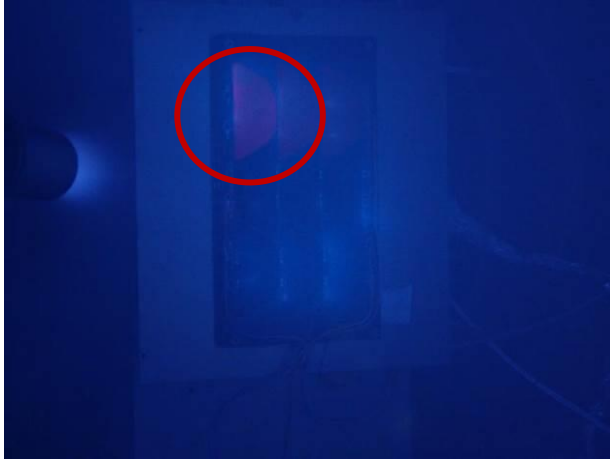
Figure 8. Glow discharges on solar array sample.
