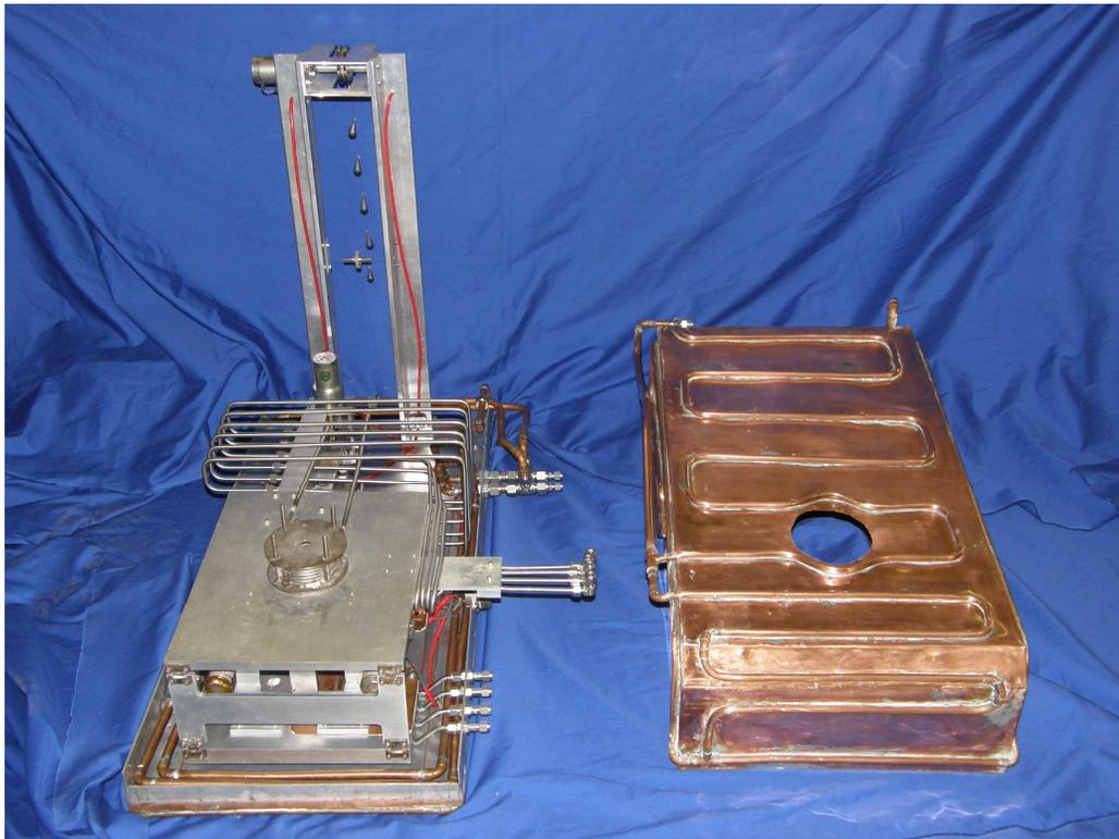
**Figure 39. (left) Thrust stand; (right) copper shroud**
