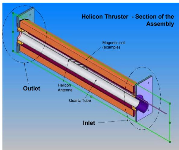
Figure 4: Diagram of the experimental helicon thruster.
