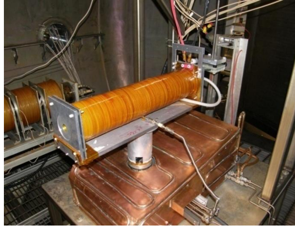
Figure 2. Medium-power helicon thruster mounted on thrust stand.
