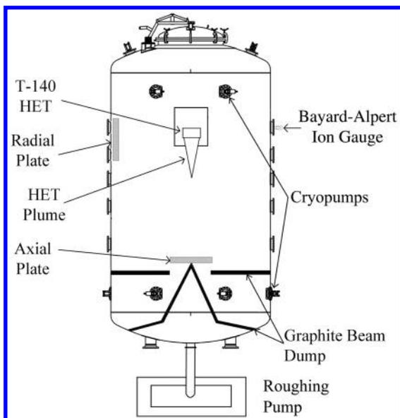
Fig. 1 Schematic of VTF-2 (not to scale).
